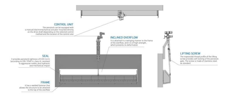
>>> FLOW SPLITTER is designed for splitting the flow (full/partial), regulating and changing the direction of flow in channels and tanks. The flow is controlled by changing the position of the penstock gate in relation to the direction of flow. Sealing gaskets are installed on the sides and the bottom of the gate to prevent leaks after closing the drain channels.
