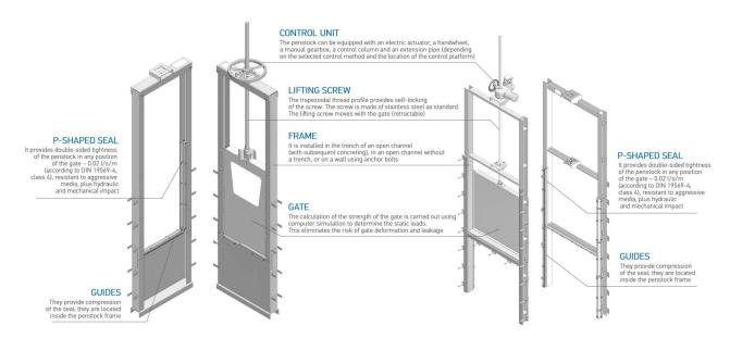
>>> STOPLOG GATES are used for temporary shutting-off during repair and installation work in gravity tanks and open channels. The gate is lowered into the frame with the help of lifting devices, providing a temporary leak shut-off of the flow during the period of repair and installation work. The gate blocks the flow in the lower position, enters the frame body through the hollow upper bar and moves down touching the side guide bars to the lower bar.
