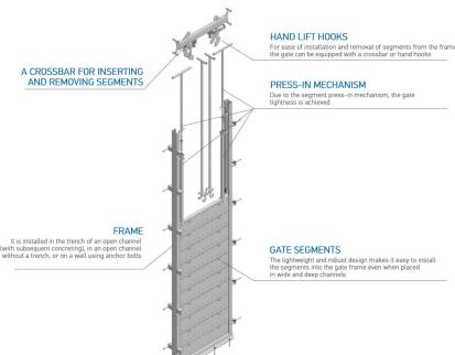
wodular stoplog gates are used for maintenance and repair of the main penstock installed nearby, for redistribution of flow in gravity tanks and open channels. The gate segments are installed in a frame mounted in the channel to temporarily block the flow. A seal is provided between the gate segments, which, in combination with the clamping mechanism, increases the tightness of the gate in the closed state.
