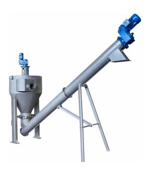
The sand conveyor is installed at an angle of 35° and is presented as a fixed enclosure assembled from sections with a rotating screw located inside of it. The round enclosure is protected from abrasion inside by wear-resistant inserts. The enclosure sections are connected by flange connections.
