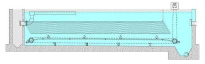
> 3-shaft scraper system for bottom sediment removal:
